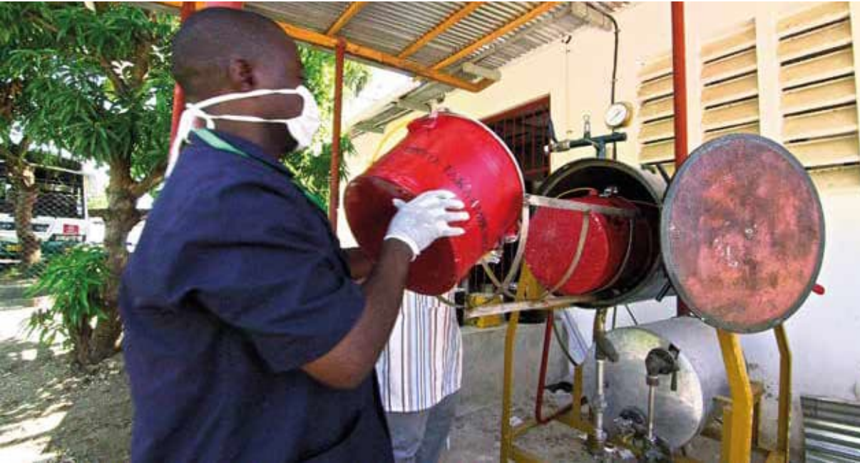
Tanzania – loading medical waste into autoclave for proper disposal
