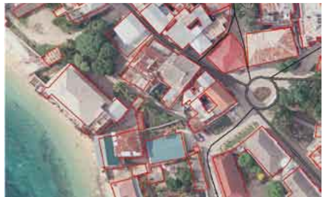
Aerial photos provided by SMOLE are used for production of updated digital maps. GIS applications are developed for land and environmental management and revenue collection.
