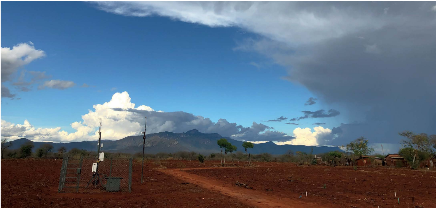
Taita Research Station of the University of Helsinki has established a station in Taita Taveta County in Kenya to measure greenhouse gas and energy exchange between atmosphere and biosphere. Photo: Petri Pellikka, 2019.
